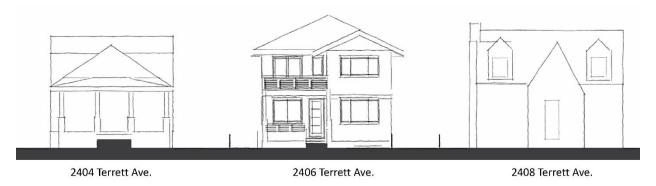
Figure 9 – Front Elevations of Proposed Dwelling with Neighboring Properties
