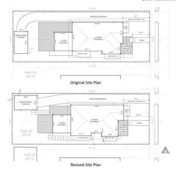
Figure 2 - Original Site Plan Proposal (Top), Final Revised Site Plan Proposal, dated October 14 (Bottom)
