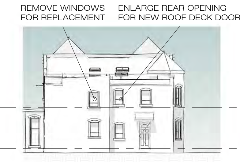
3 Existing - Rear Elevation A101 1/16" = 1'-0"
