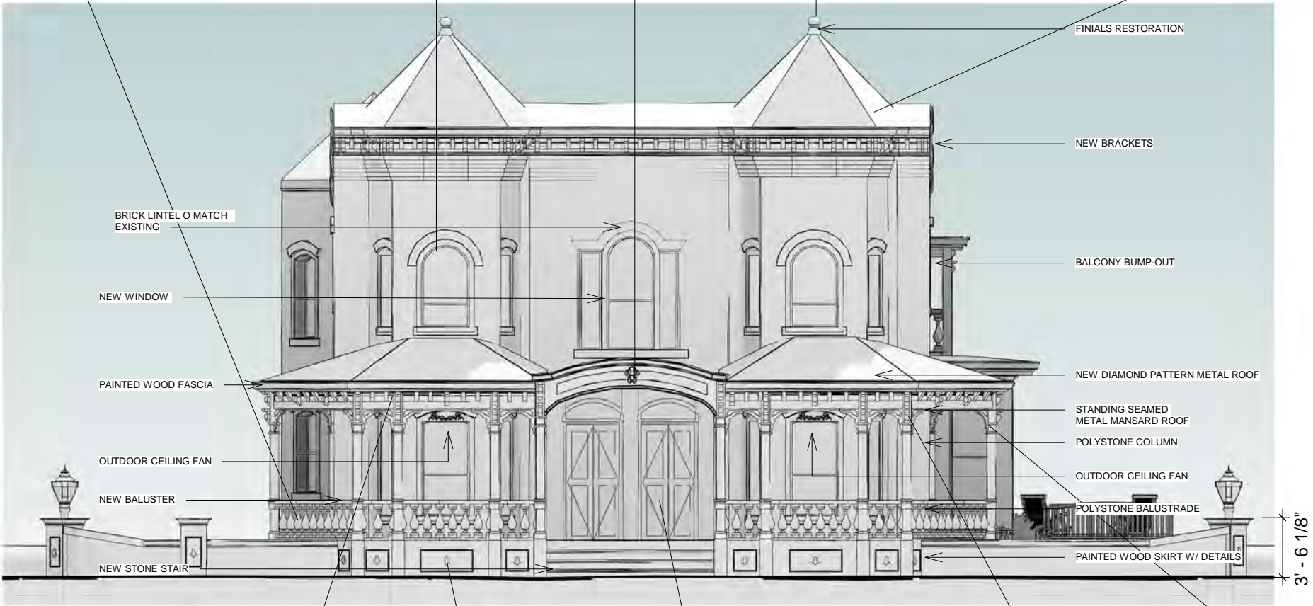
1 commercial front porch elevation A105 1/8" = 1'-0"
