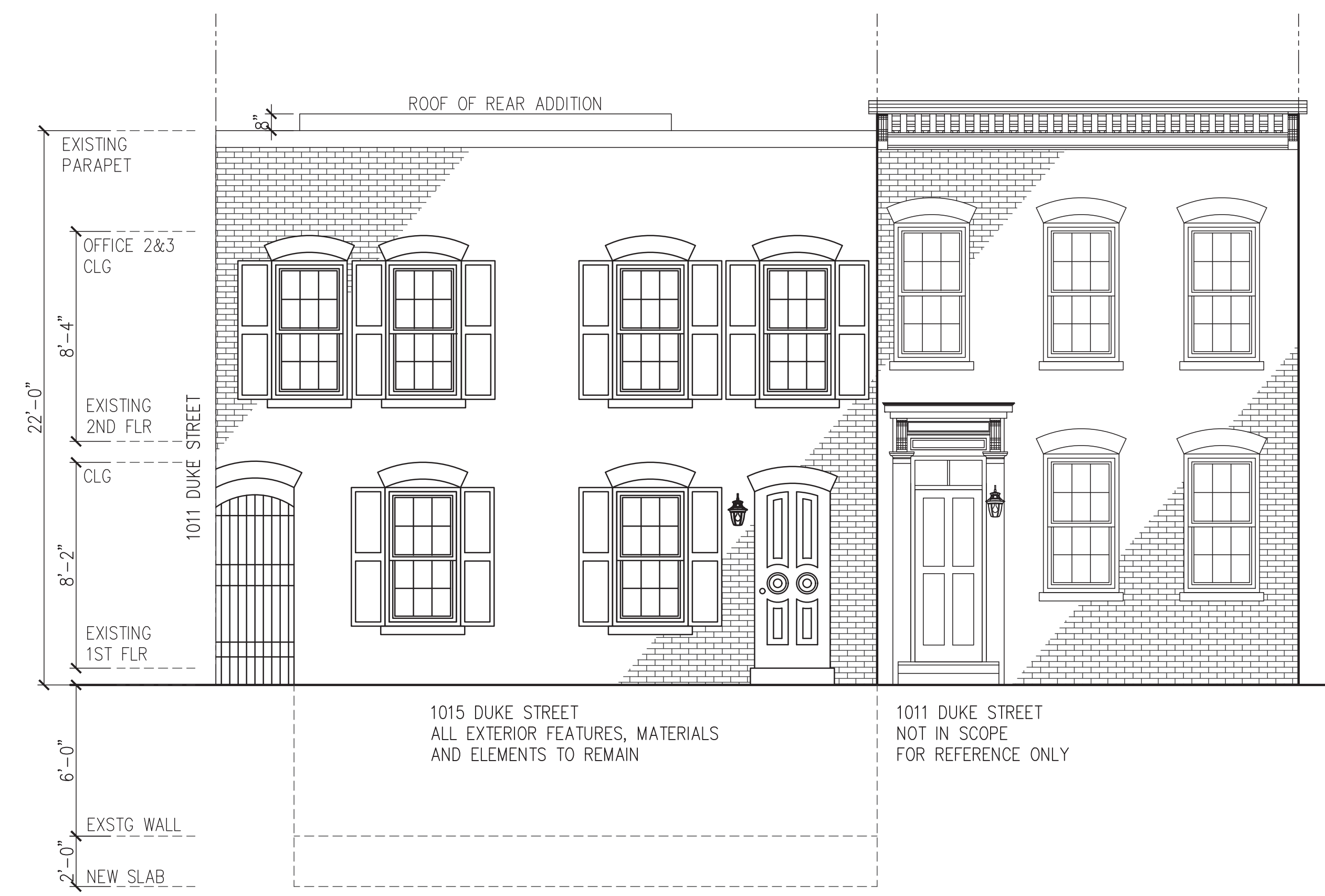
A PROPOSED SOUTH ELEVATION (FRONT)
