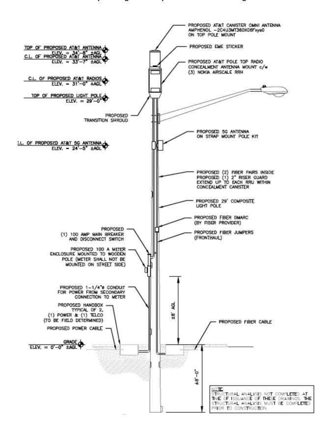
A-12: Composite Light Pole Replacement with 5G Configuration
