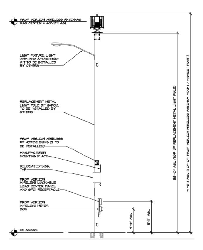
A-8: Metal Light Pole Replacement with 4G/5G Configuration
