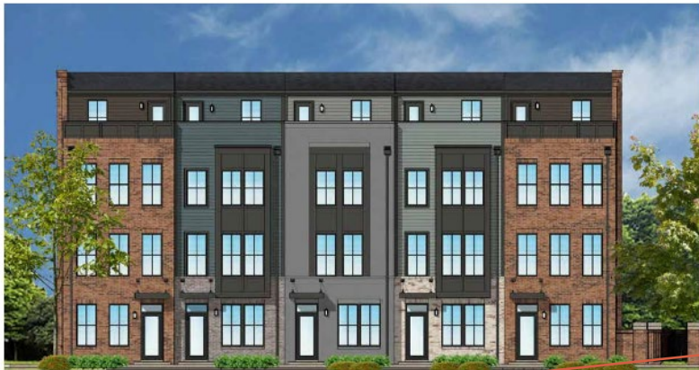
5-UNIT & 6-UNIT FRONT ELEVATION FULL BRICK FRONTS AT BUILDING ENDS OTHER UNITS PARTIAL BRICK AND SIDING
