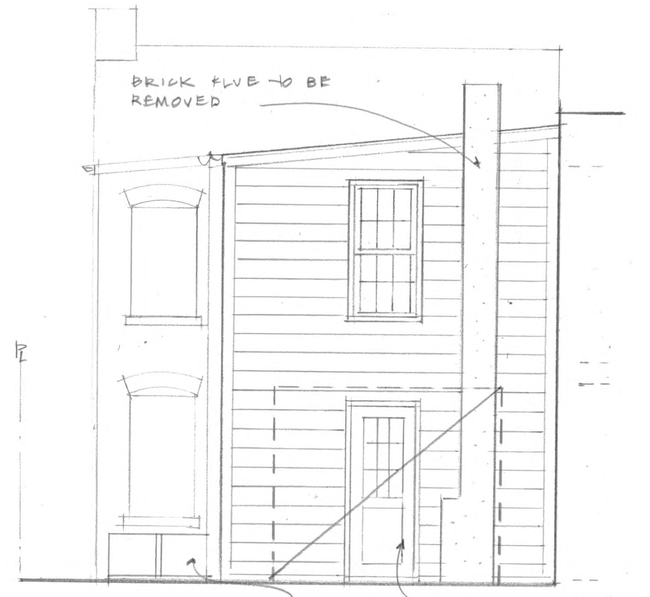
2 REAR ELEVATION - EXIST & DEMO
