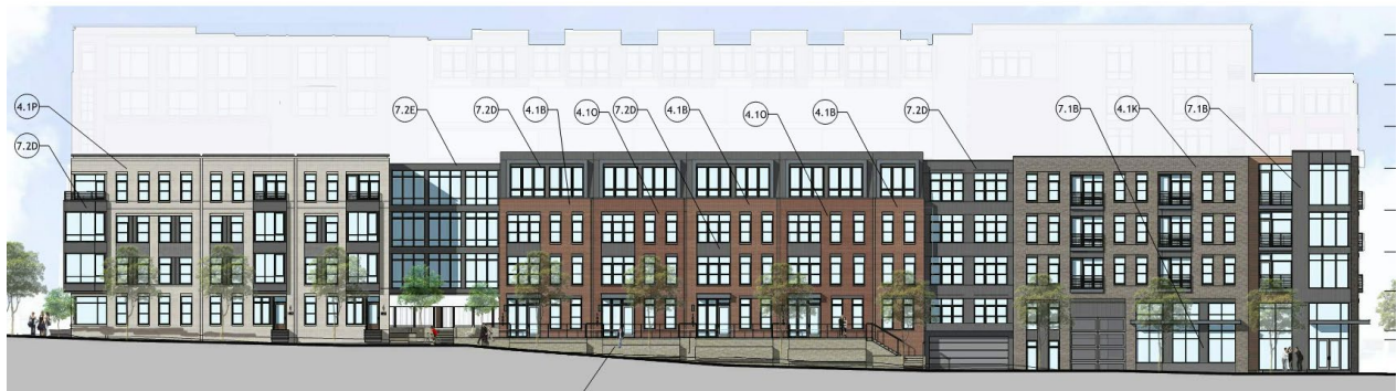
Figure 14: East (S. Alfred Street) elevation of Block 4 showing the grade change between a low point of the block (right) with a higher point of the block (left). Note the elevated walkway entrances in the middle of the block.
