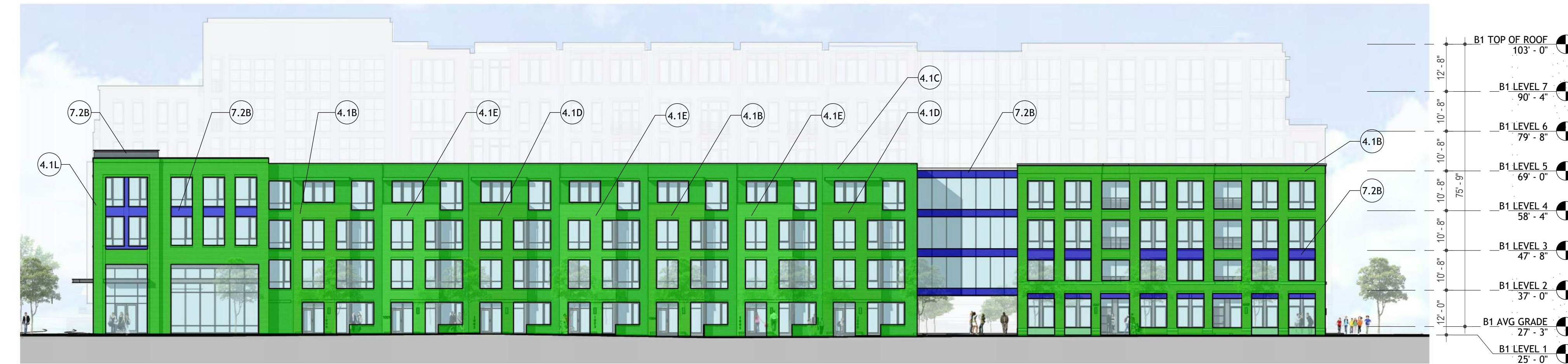
4 BLOCK 1 - EAST ELEVATION - S. ALFRED ST. - MATERIALS EXHIBIT A0.10A/A1.12E 1" = 20'-0"
