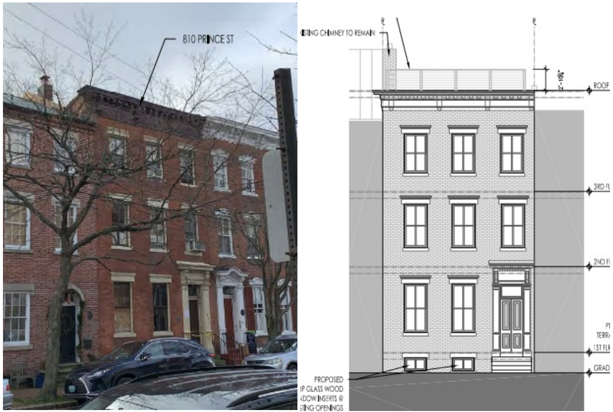
Figure 5: The rendering on the right indicates that the metal railing will extend approximately halfway up the existing chimney. The photo on the left indicates that the chimney is barely visible from the street.
