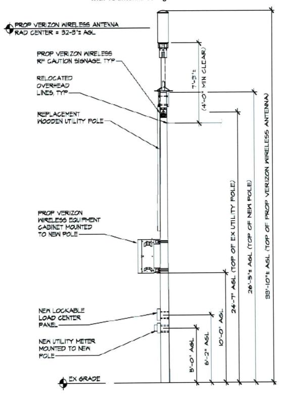
A-2.1: Wood Utility Pole Replacement and Stand-Alone Pole with 4G antenna Configuration
