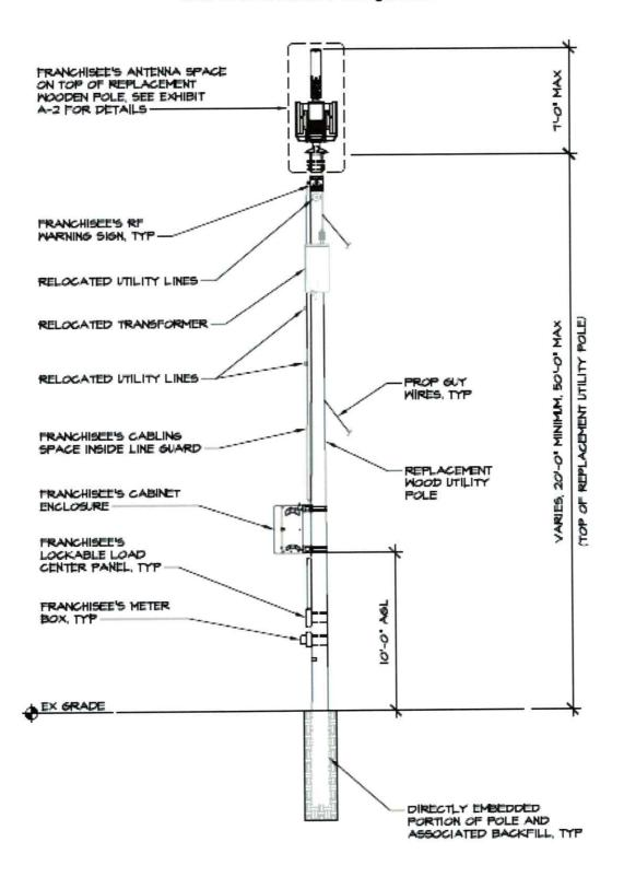
A-2: Wood Utility Pole Replacement and Stand-Alone Pole with 4G antenna Configuration
