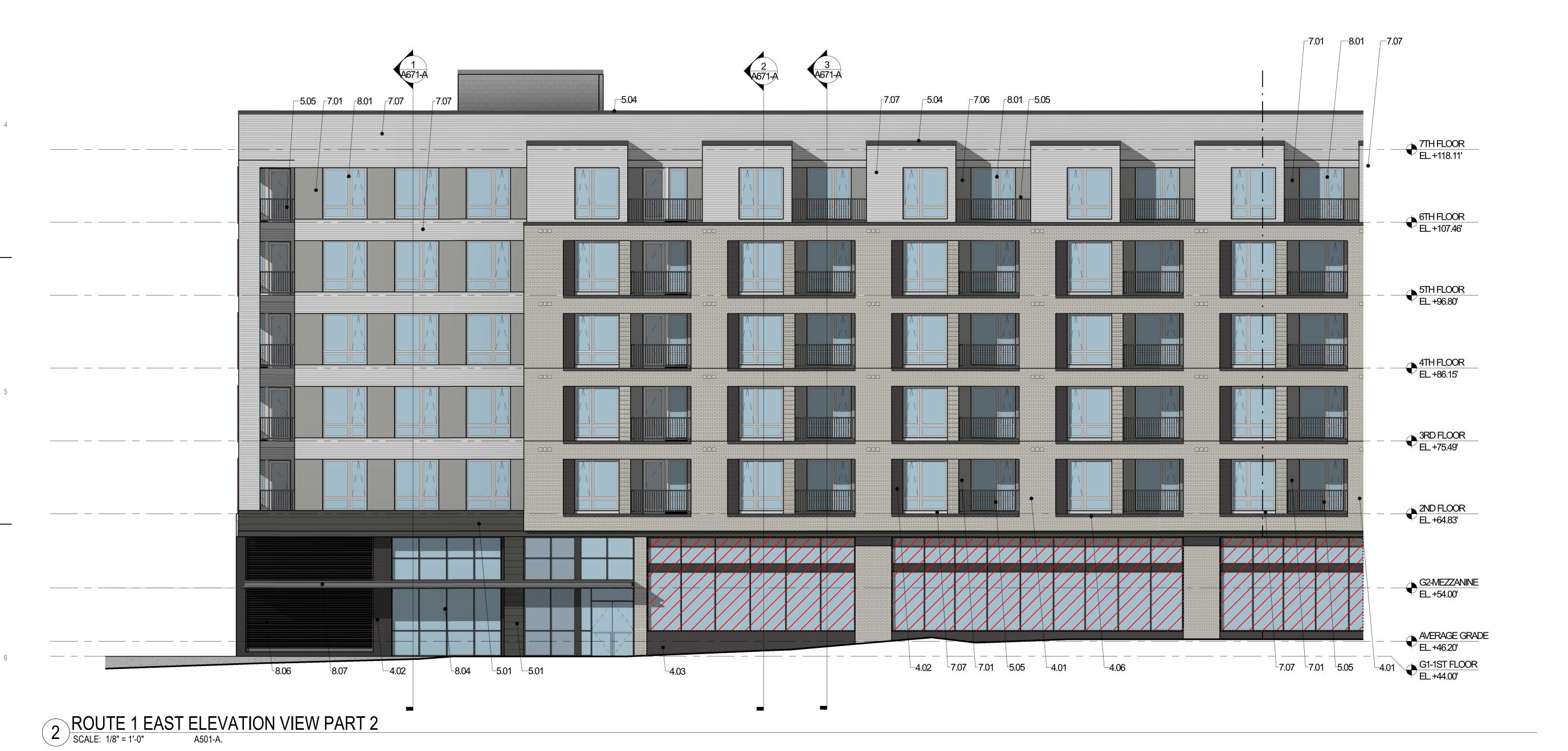
Retail storefront shown in elevations at tenant openings are example of potential final condition. Openings will be temporarily enclosed with painted plywood cladding with graphics, or similar, as required by code for certificate of occupancy. See precedent images on this sheet for possible temporary storefront treatment. Prior to construction bond release, permanent storefront will be constructed in retail bays which have not yet submitted for building permits for tenant fit out.
