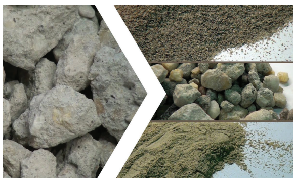
Figure 23. Concrete can be crushed and reused for other applications
