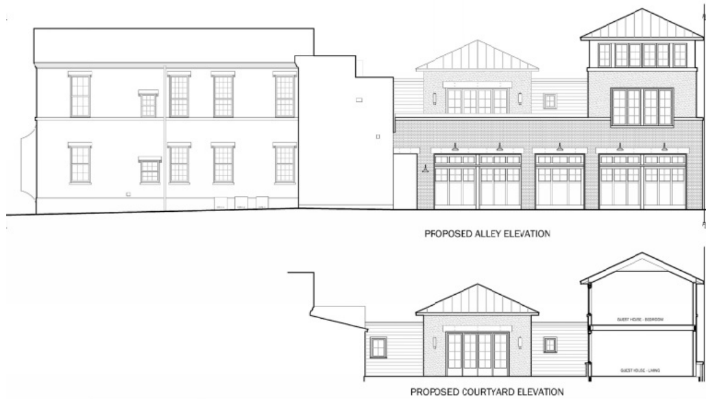
Figure 4: Proposed north elevation. Note that westernmost (right) roof looks taller than that of the 1818 building; the applicant intends to lower the new roof to the same height as the original.
