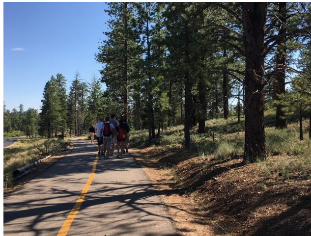
Figure 45: A section of trail in Bryce Canyon with adequate recovery zones, vertical clearance, and separation from the road
