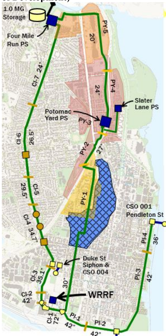
Figure 1: Existing Sanitary Sewer Infrastructure (Design Based on 6.4 Million Square Feet of Development)
