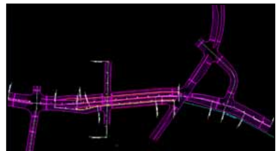
Figure 5-7. Frontage roads alternative. Alignment of Duke Street and New High Street with frontage roads along Duke Street at plaza level and through traffic operating at a lower level at the existing grade of Duke Street.
