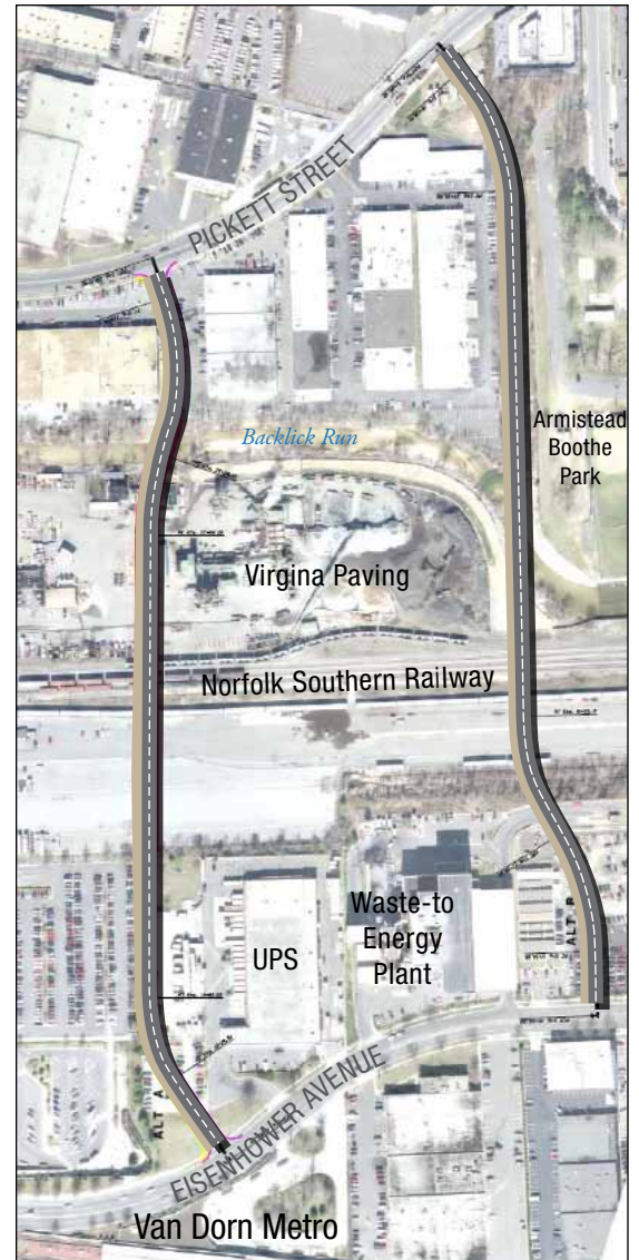
Figure 5-16. Alternative routes for connecting bridges between Pickett Street and the Van Dorn Street Metro Station. The western alignment would link pedestrians to the existing concourse under Eisenhower Avenue and connect directly to the new north-south street through Pickett Place. The eastern alignment is adjacent to Armistead Boothe Park and would provide more convenient access from Cameron Station and other areas to the east, and could be designed to connect directly to Pickett Place Main Street. The eastern alignment could join Cameron Station Boulevard as an alternative to directly intersecting Pickett Street. These alternative alignments are conceptual and not final. The final location will be determined at a later date after further study.
