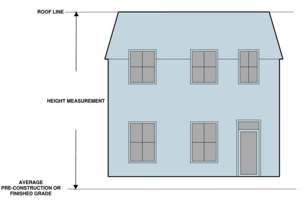
(D) Dormers. In the case of dormers, height shall be measured to the midpoint between the dormers eaves and the ridge. For buildings in the R-20, R-12, R-8, R-5, R-2-5, and single-family and two-family dwellings in the RA and RB zones, not including property located within the Old and Historic Alexandria and Parker-Gray Districts, height shall be measured to the midpoint of the dormers if the total width of all dormers is more than 30 percent of the horizontal width of the roof.
