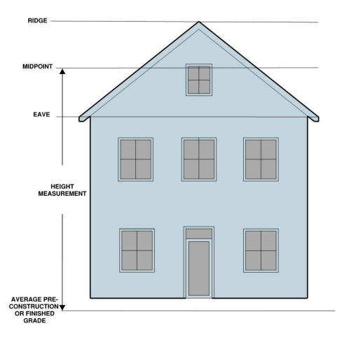
(2) For purposes of establishing the setback ratio on the gable end of a building with a gable roof, height shall be measured to the midpoint between the eaves and the ridge.
