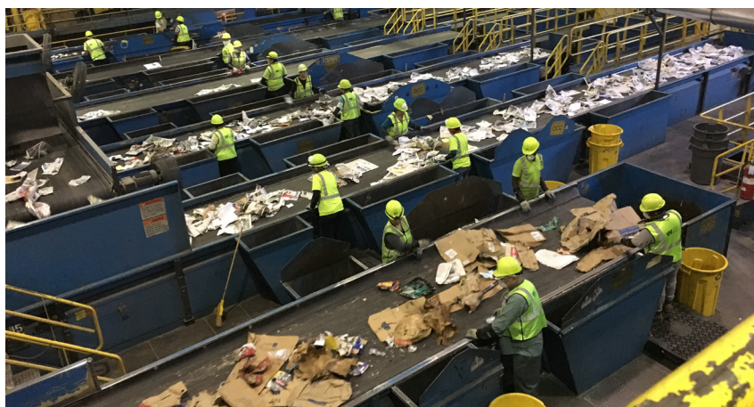
Figure 11 Recyclables being sorted at a Material Recovery Facility
