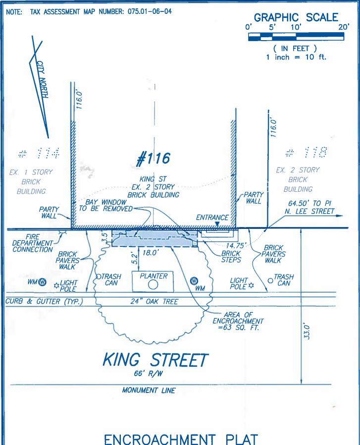
SHOWING AREA OF ENCROACHMENT FOR WINDOW (PASS THRU SERVICE) ON THE PROPERTY LOCATED AT
