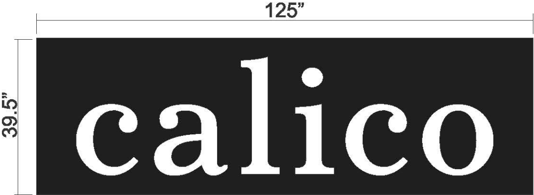
FRONT ELEVATION - Sign Type (A)(QTY:1) Exterior Illuminated Awning - Sunbrella Fabric Scale: 1/2" = 1' (34.4 SQFT)
