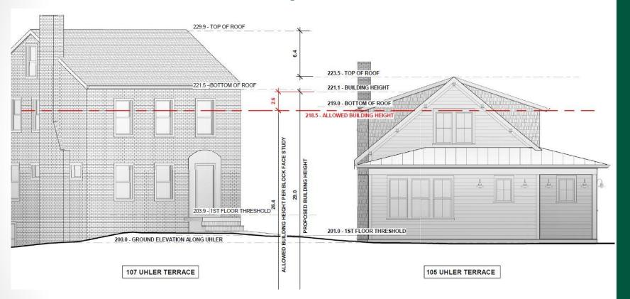
Height at front elevation of 21.10 Ft. is less than block face average of 22.00 Ft.
