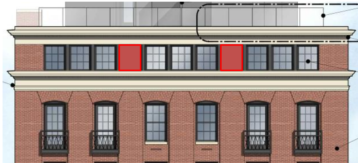
Figure 3. Proposed attic story with continuous ribbon window. The red boxes suggest where the false windows could be eliminated and the brick retained.
