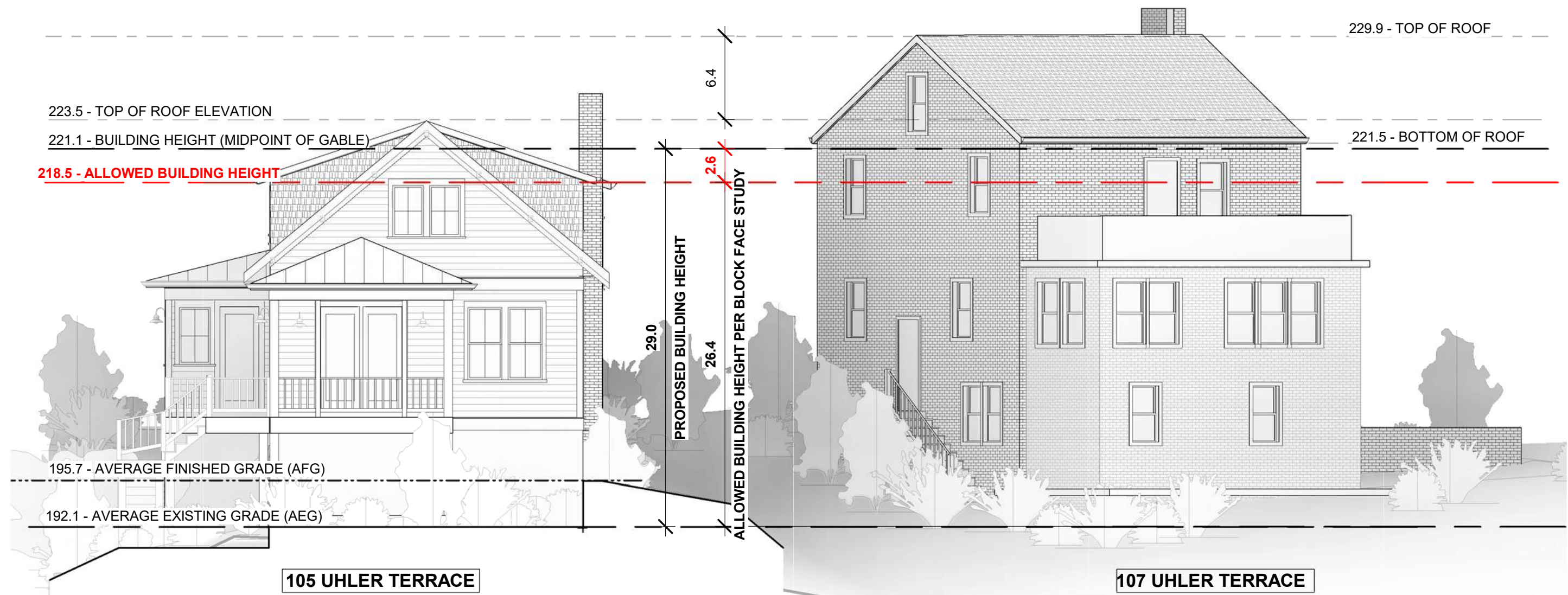
1 EAST (REAR) ELEVATION - HEIGHT COMPARISON TO 107 UHLER 1/8" = 1'-0"
