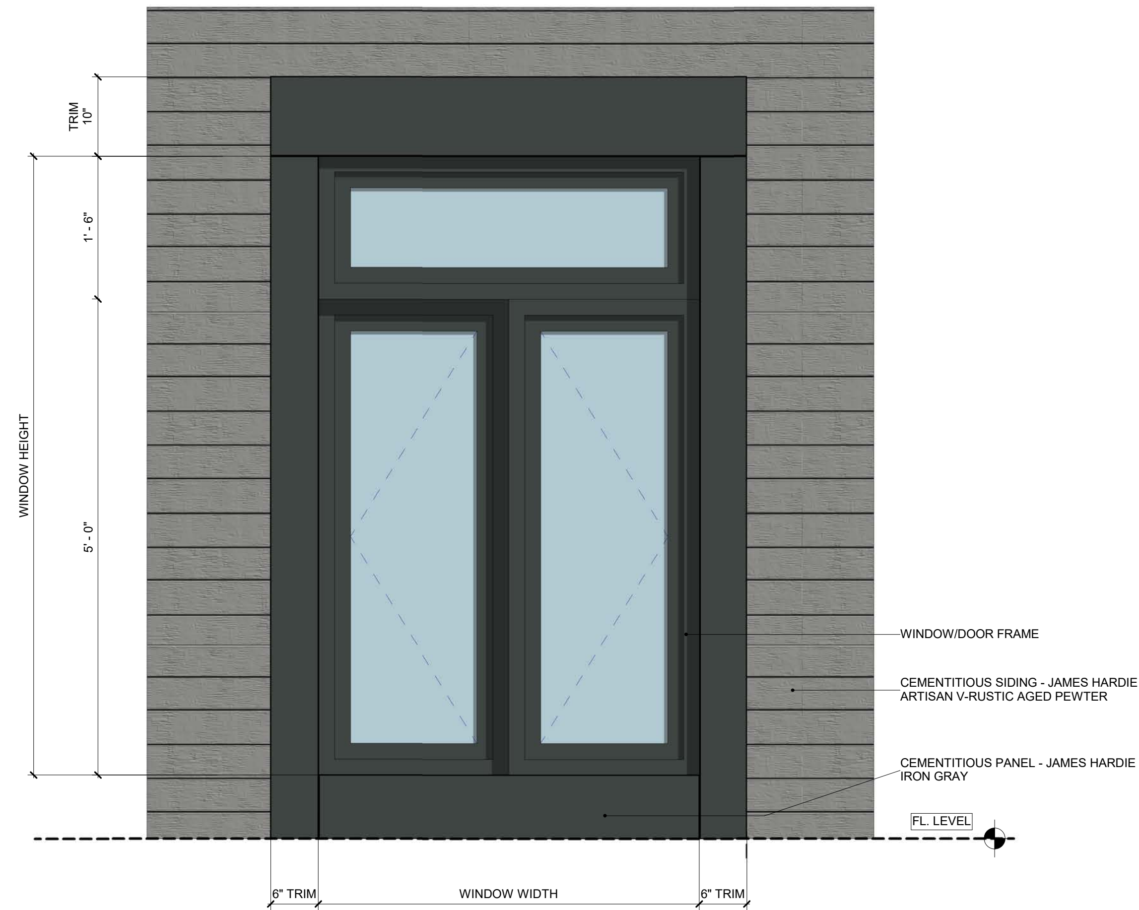
DOUBLE CASEMENT WINDOW AT HARDIE SIDING 2 1" = 1'-0"
