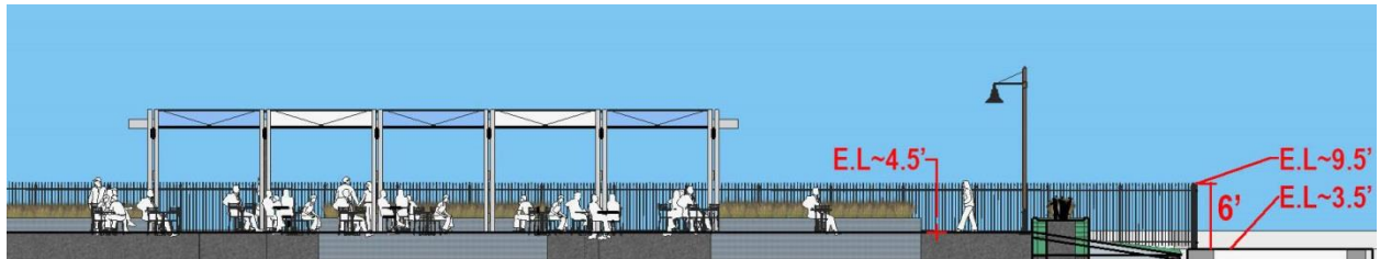
Figure 5: Site section created by City staff showing the proposed fence behind covered seating area, looking north. The existing pier platform is on the right.
