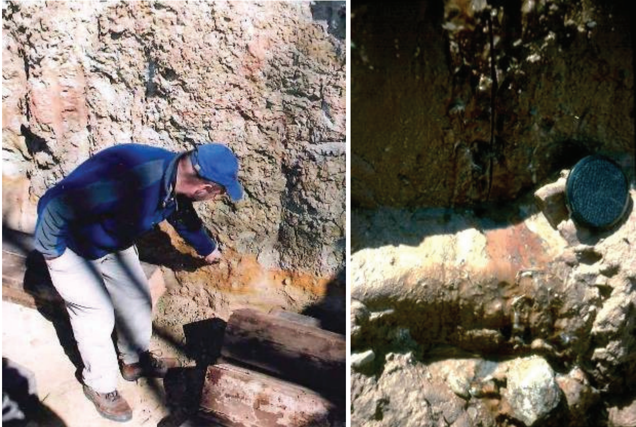
Figure 3. Left: Heavily fractured Arell clay exposed on a hillside in the Hospital escarpment. Photo by Rod Simmons. Right: Ground water discharging from a fracture (to the left of lens cap) in otherwise nearly impervious clay. When the hydrostatic pressure inside the fracture increases, such as during heavy rains or through human alteration of near-surface hydrology, the fracture dilates. When this process occurs on hillsides, it may lead to a loss of frictional strength sufficient to cause the slope to fail along the fracture. Photo by Tony Fleming.
