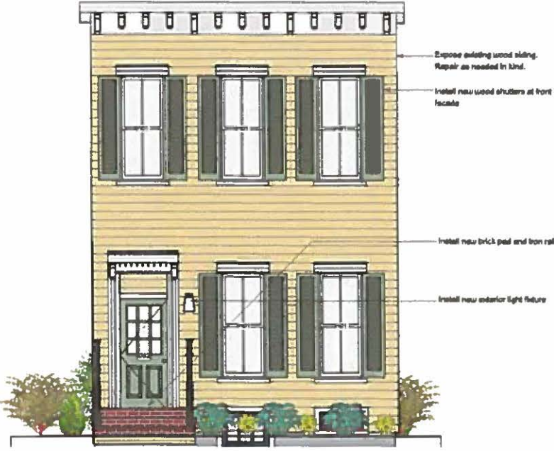
Proposed Front Elevation Scale 1/8"=1'0"
