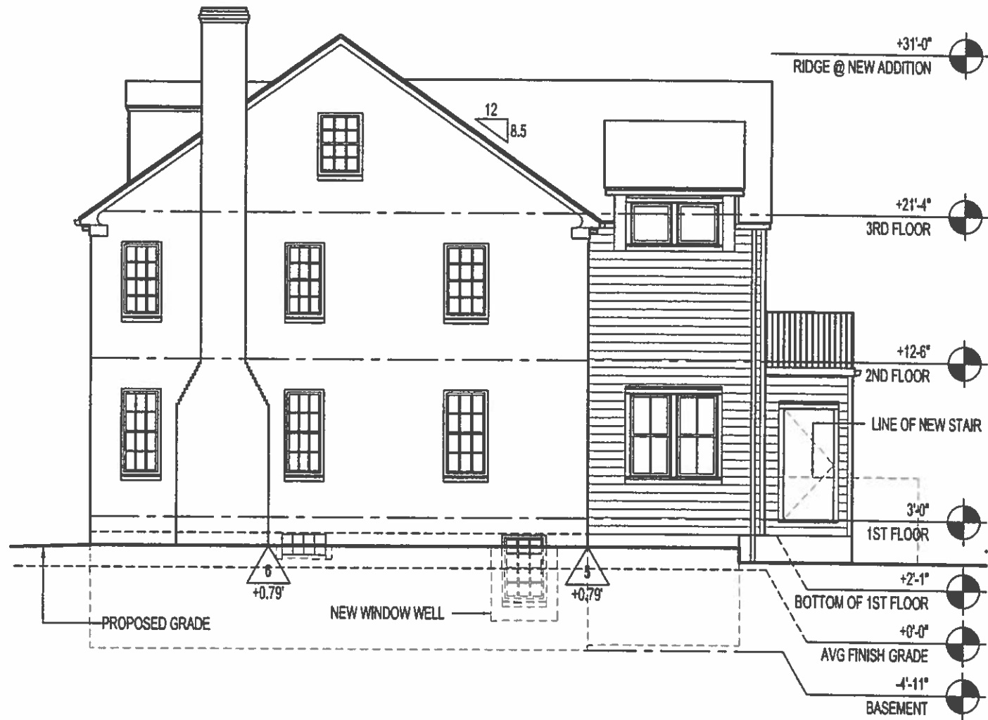
2 NEW SECONDARY FRONT / SOUTH ELEVATION 1/8" = 1'-0"
