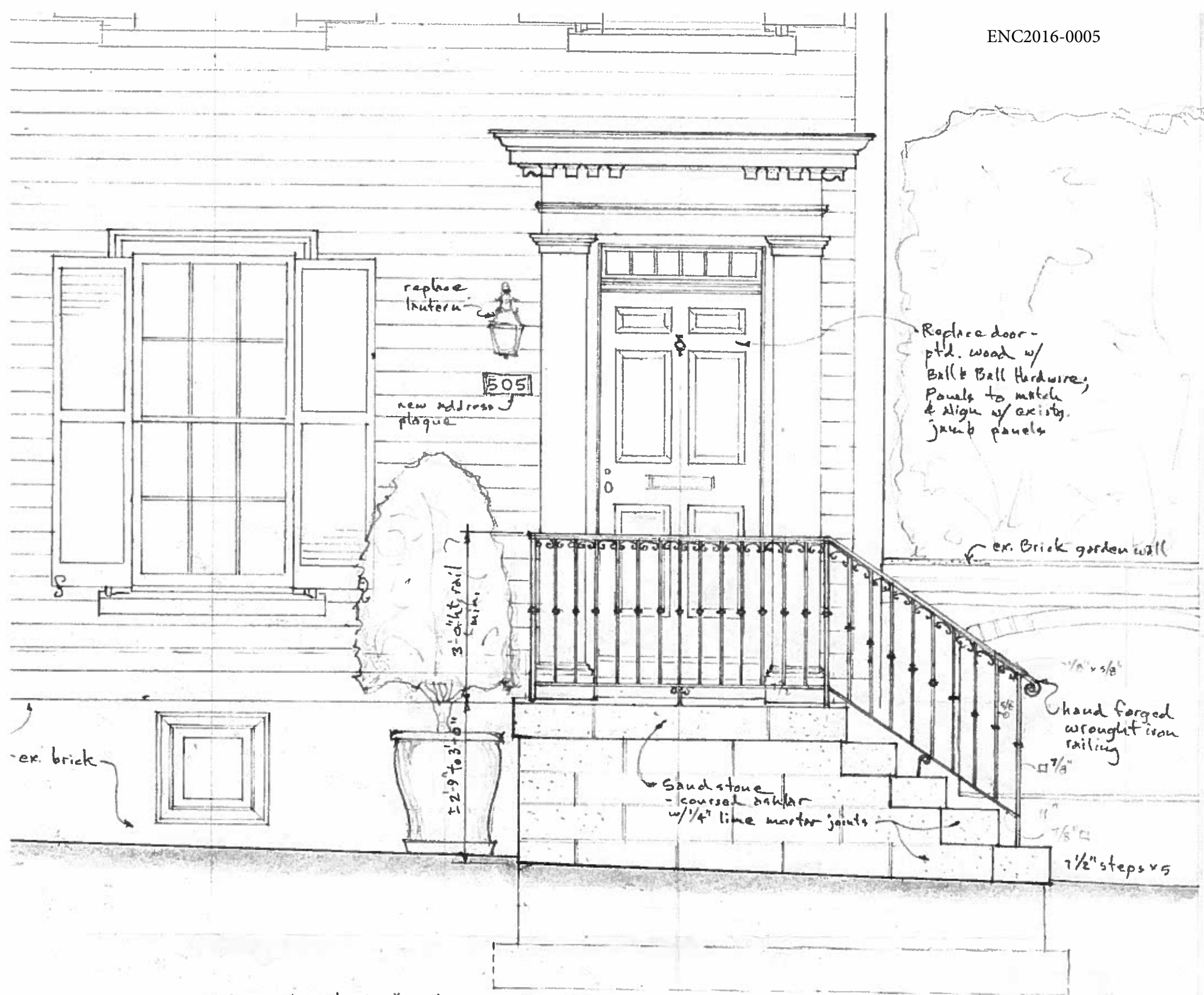
East Elevation of Entry 1/2" = 1'-0"
