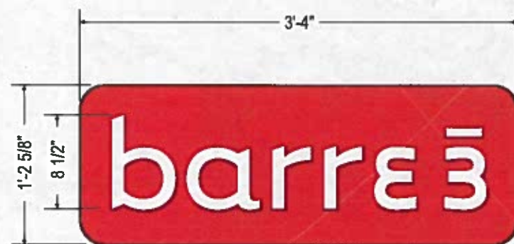
S/F FLAT WALL SIGN WITH FLAT CUT OUT LETTERS SCALE: 1" = 1'-0"
