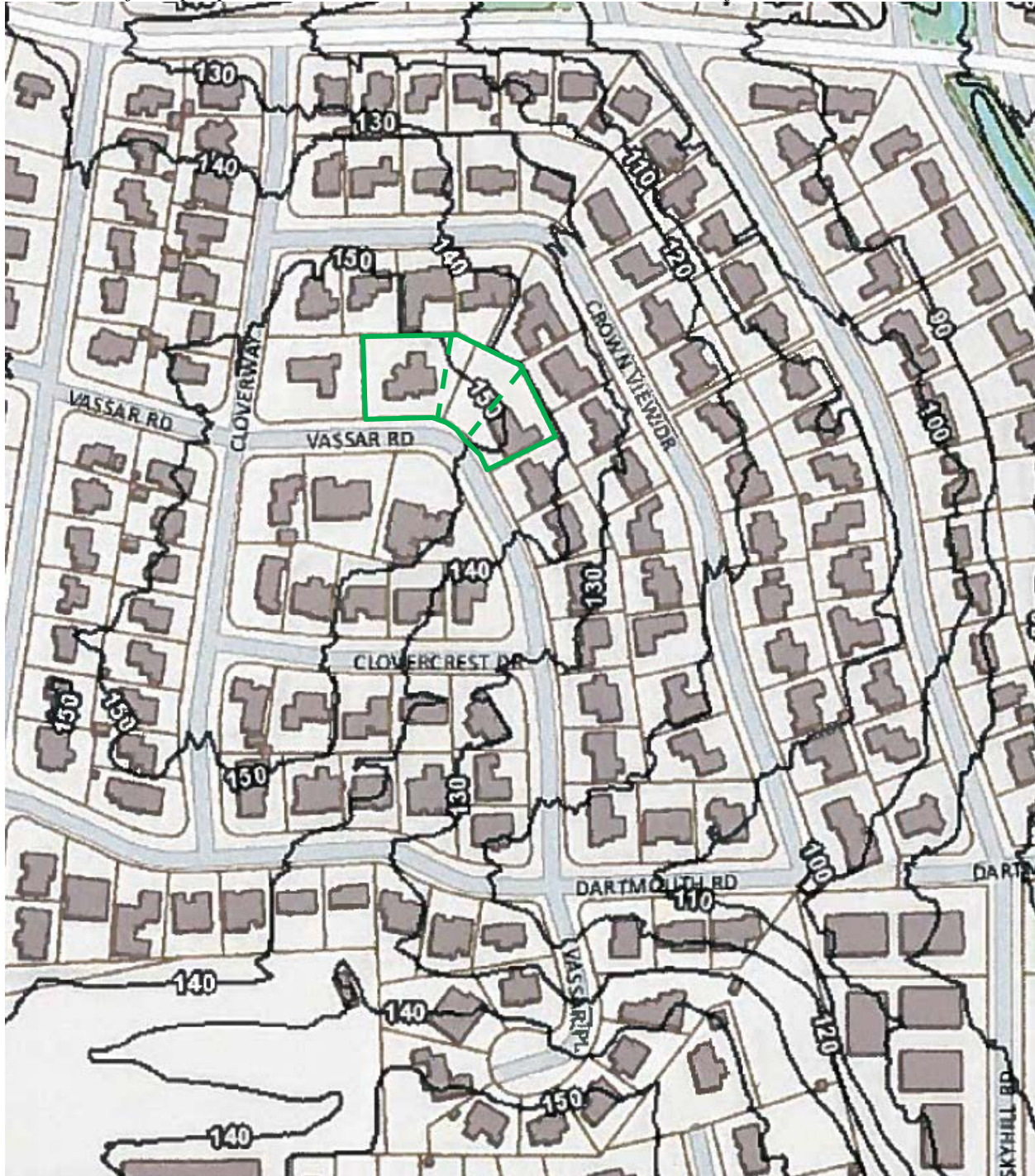
Figure 5: Topography of the Clover Neighborhood. The highest areas are to the south and southwest of the proposed subdivision lots and at the southern end of Vassar Place.
