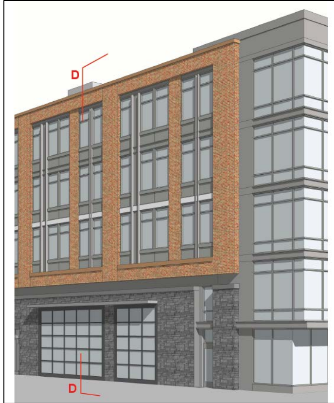
Figure 2. West elevation of Building 1 showing stone base, garage/loading doors and applied brickwork.
