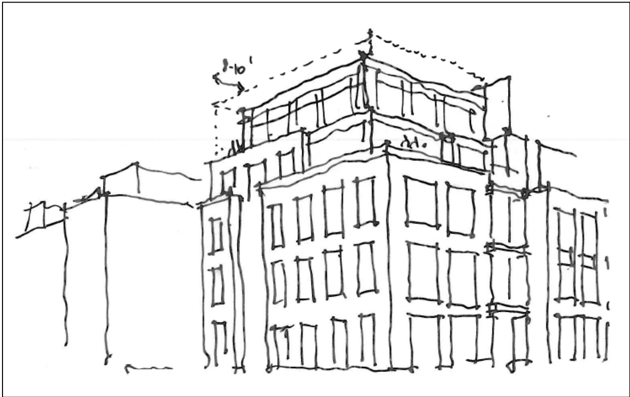
Figure 3. Schematic massing sketch showing more pronounced upper floor set backs at corner of South Union and Wolfe streets. Dashed lines illustrate submitted building volume.
