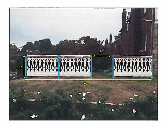
Fence is 25 linear feet and will be 3' 6" high to comply with Alexandria codes. The gate will be between 30" and 36" style will be similar to the slats.
