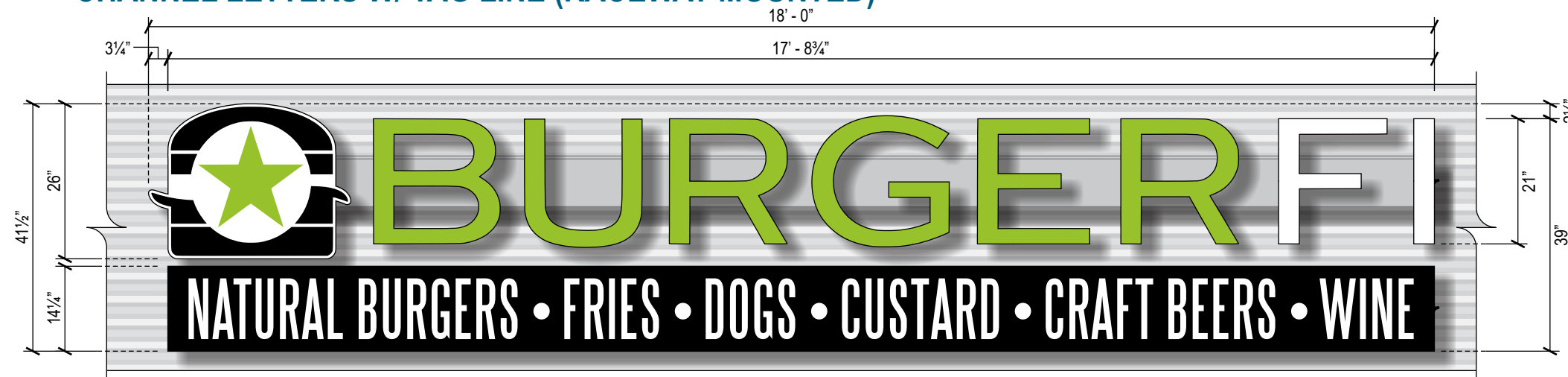
7.1 CHANNEL LETTERS (RACEWAY MOUNTED) - CL-21-RW-TAG SCALE: 1/2" = 1'-0"
