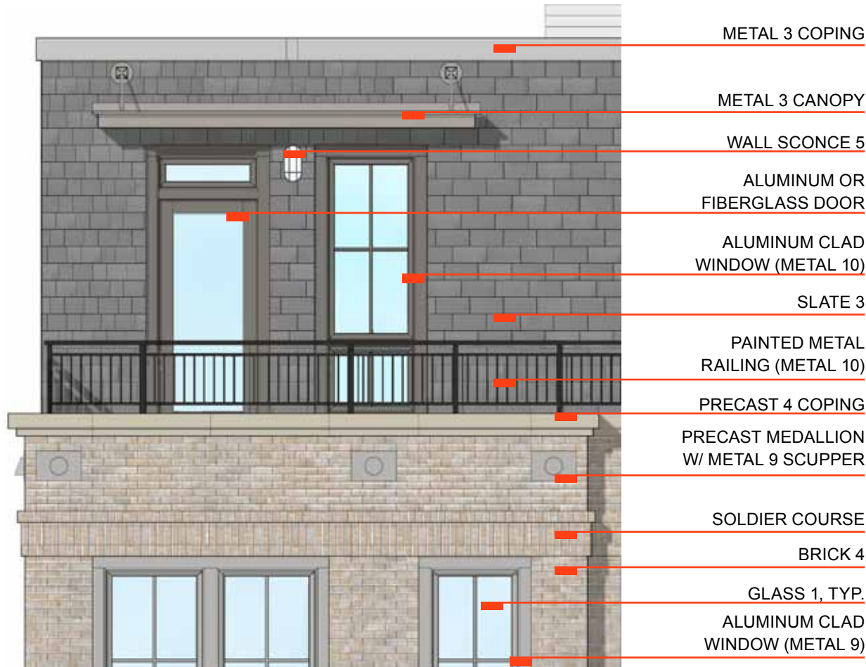
PARAPET WITH SCUPPERS AND GUARDRAILS
