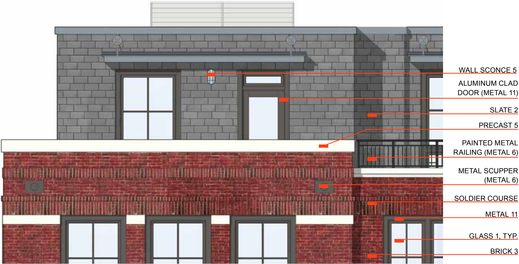
PARAPET WITH SCUPPERS AND GUARDRAILS
