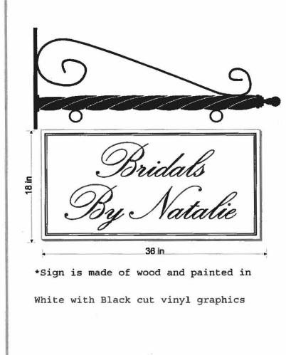
36" iron scroll bracket installed into motar joints using lead anchors and 5" x 3/8" lag bolts install sign so bottom of sign is 9 ft. from sidewalk sign bracket blade sign 210 1.8  $\cap$
