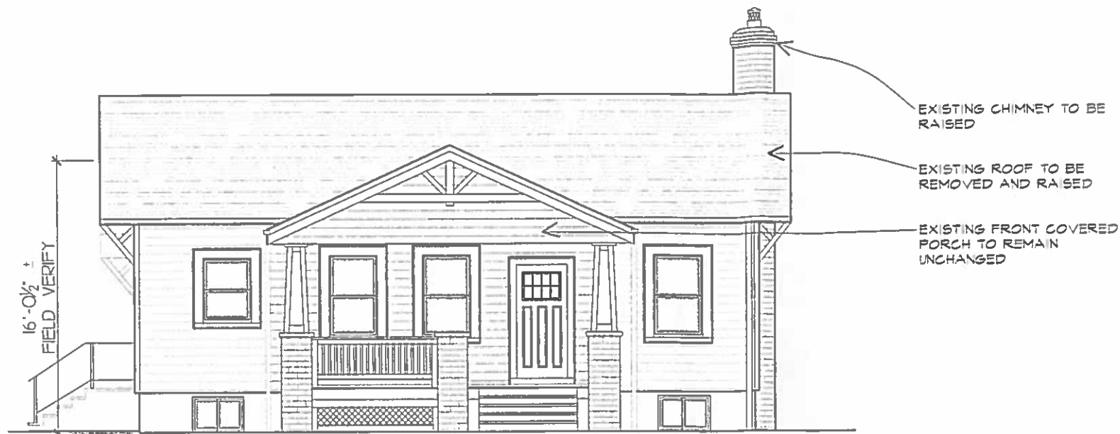
(A) EXISTING FRONT SOUTH ELEVATION 1/8"=1'-0"
