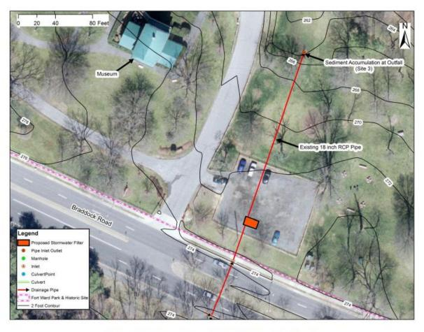
Figure 6: Proposed Stormwater Filter Concept Design
