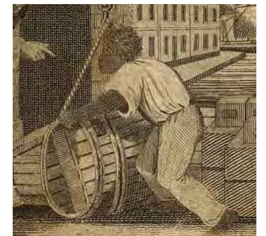
A tobacco hogshead was used in British and American colonial times to transport and store tobacco. It was a very large wooden barrel. A standardized hogshead measured 48 inches (1,219 mm) long and 30 inches (762 mm) in diameter at the head (at least 550 L or 121 imp gal or 145 US gal, depending on the width in the middle). Fully packed with tobacco, it weighed about 1,000 pounds (454 kg).
