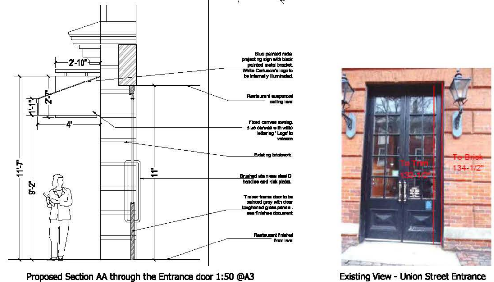
Proposed Section AA through the Entrance door 1:50 @A3
