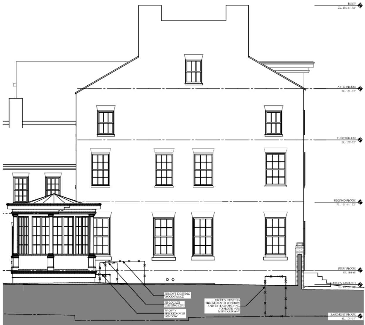
Figure 1: East elevation showing area of exterior wall to be removed
