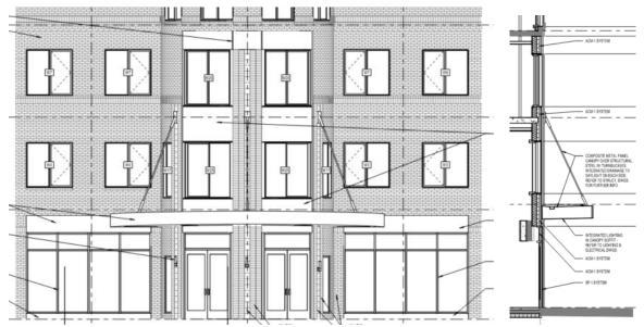
Figure 3: Proposed elevation and section at building entry showing canopy and metal panels
