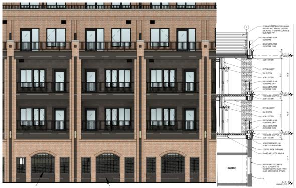
Figure 5: Proposed enclosure of Fayette Street above grade parking, elevation and section
