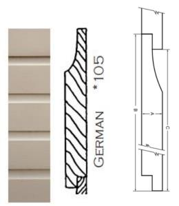
Figure 4: Typical German siding (left) & Proposed Cove/Dutch Lap siding (right)
