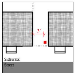
Townhouse with no setback from the property line but with a side yard or alley providing 3' clearance after installation of the meter.
