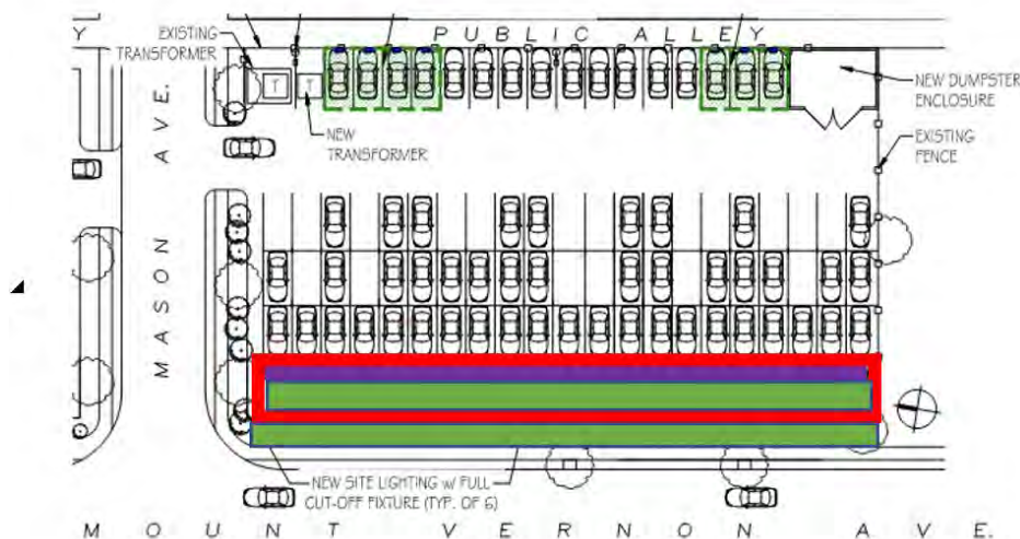
Figure 10: Twenty-one parking spaces, outlined in red, are recommended for removal and for replacement with open space at 1605-1611 Mount Vernon Avenue. Approximate areas recommended for open space and landscaping are shown in green and an addition of a decorative four-foot fence or wall mural is identified in purple.
