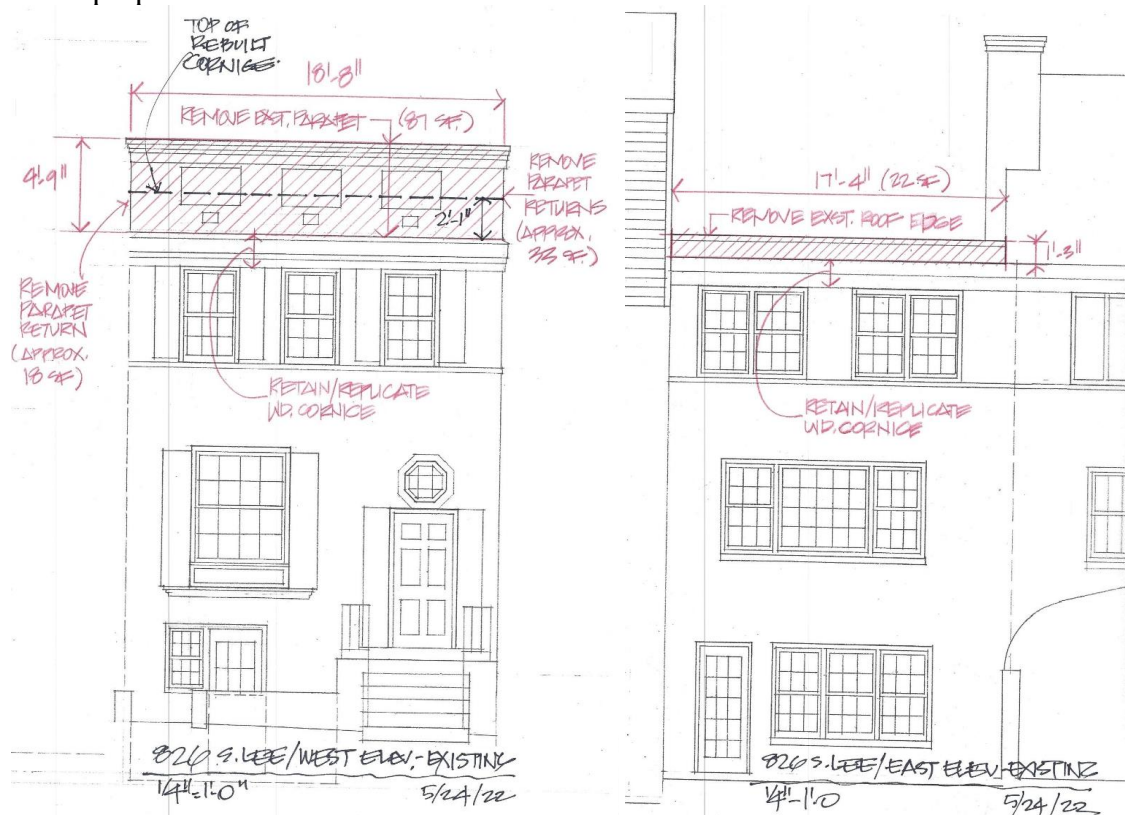
Figure 1: Proposed demolition at west and east elevations
