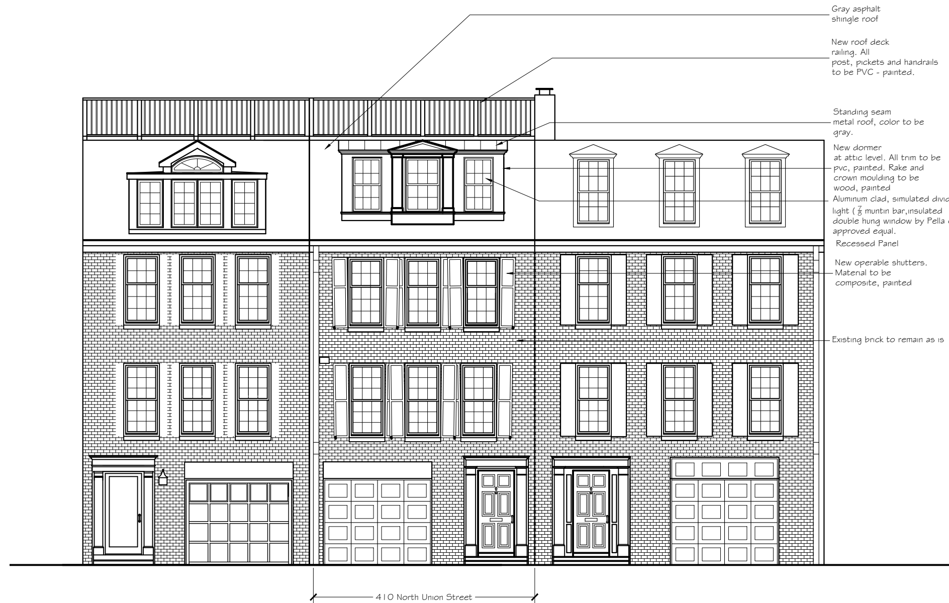
① Proposed East Elevation SCALE: 1/8" = 1'-0"
