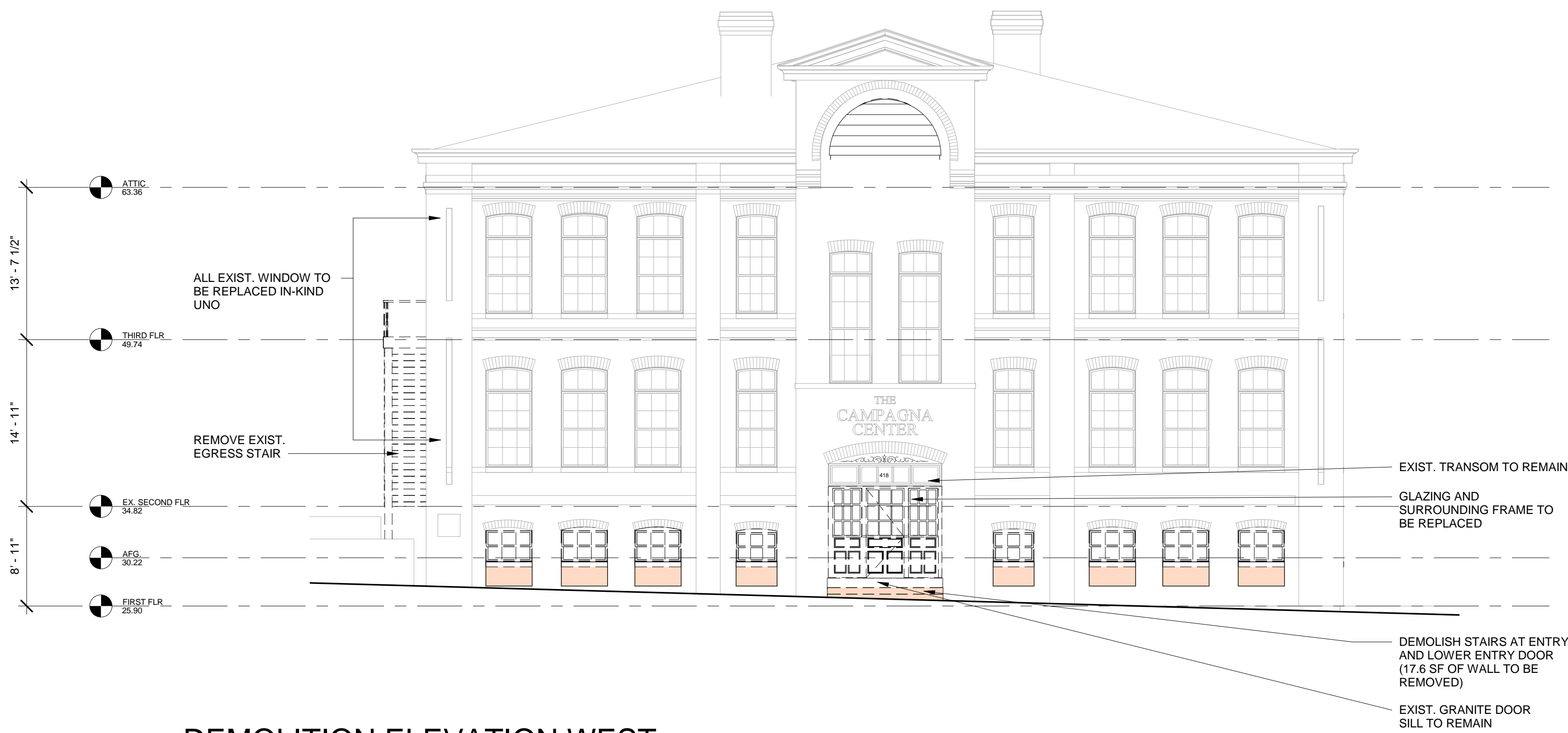
1 DEMOLITION ELEVATION WEST 1/8" = 1'-0"
