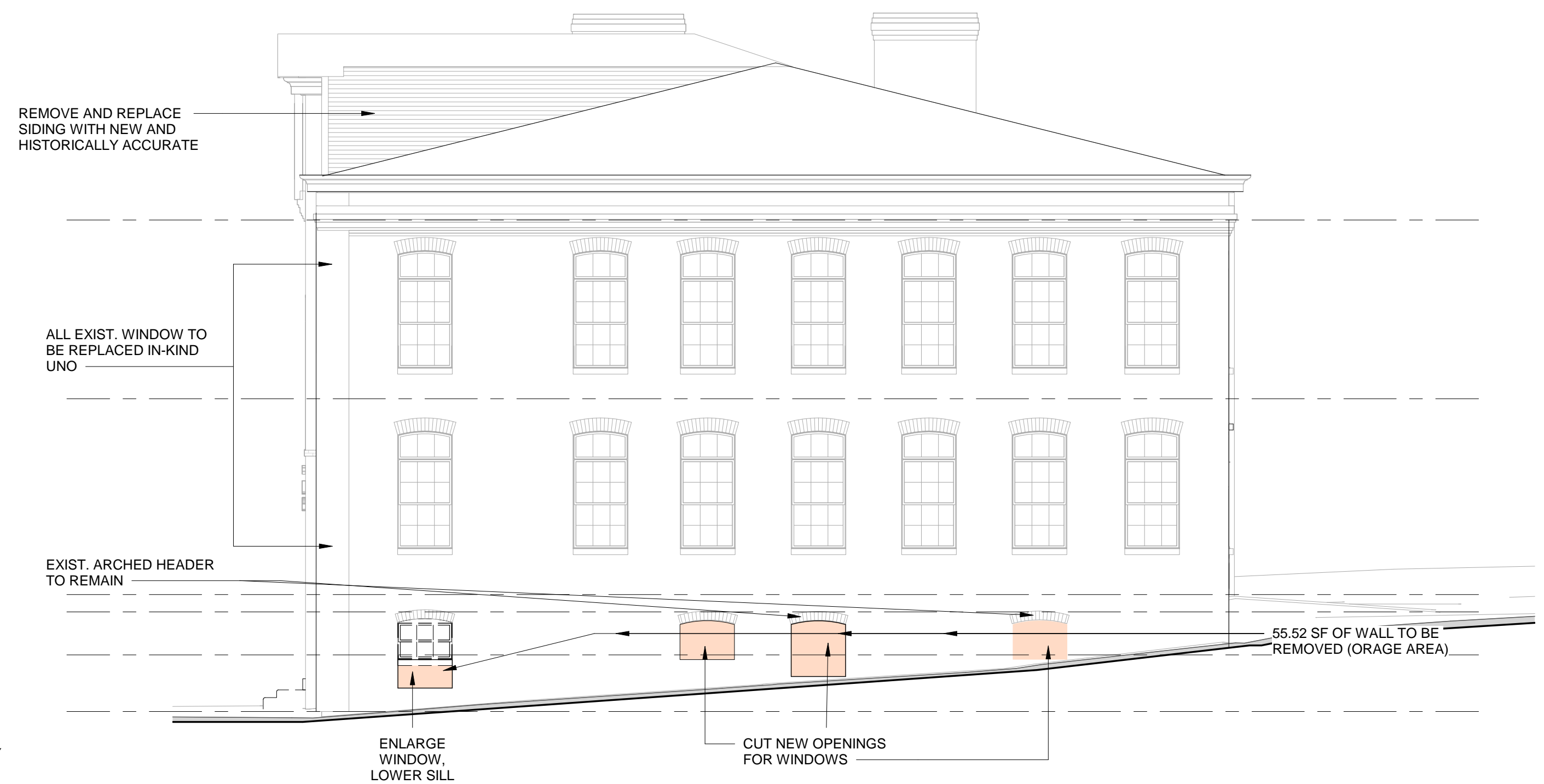
2 DEMOLITION ELEVATION SOUTH 1/8" = 1'-0"
