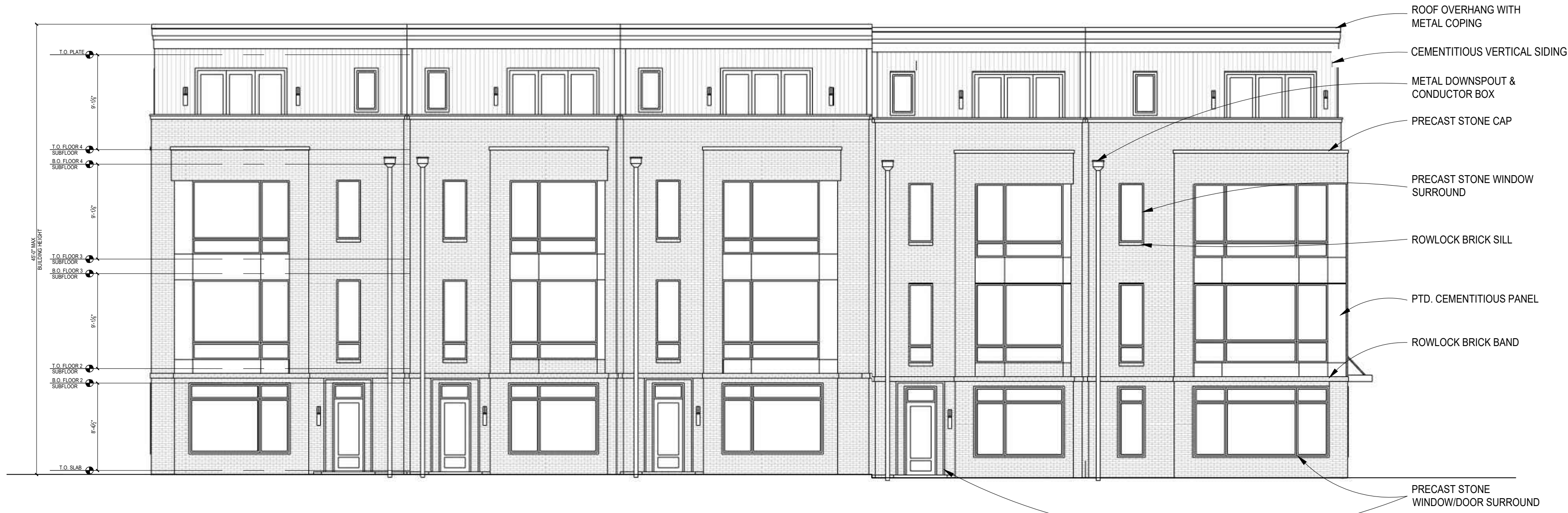
1 FRONT ELEVATION Scale: 1/8"=1'
