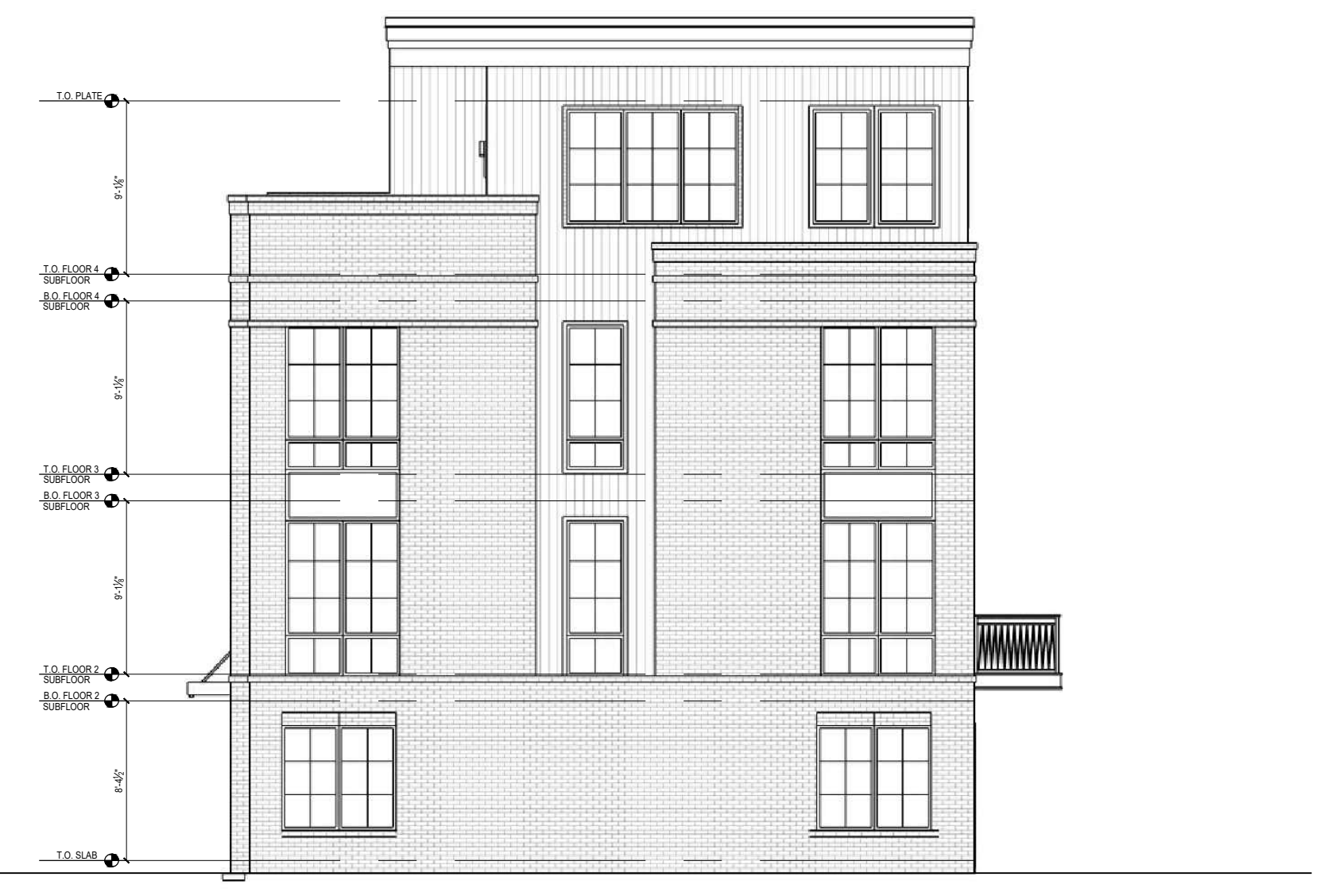
2 RIGHT SIDE ELEVATION Scale: 1/8"=1'
