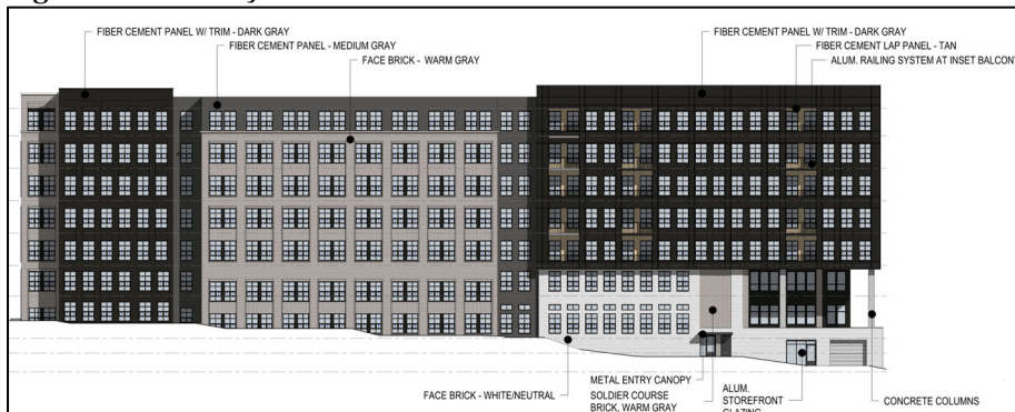
Figure 6: East Façade with materials
